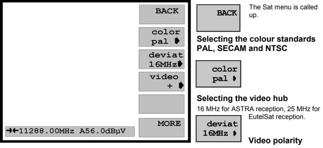
video + 🖡 Switch-over of the video polarity between positive and negative.
